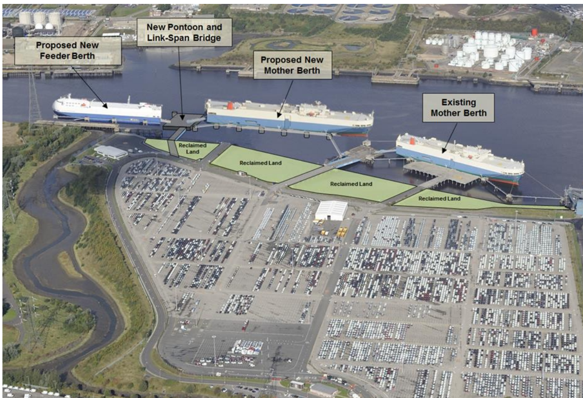
Figure 2-2: Reconfiguration of Car Terminal Berths
